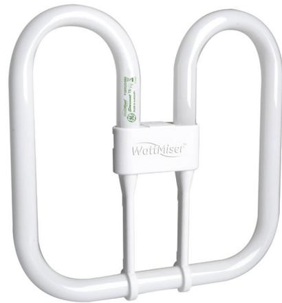
New 2D™ Watt-Miser™ lamps are energy saving compact fluorescent tubes formed into a “2D” shape. All types are available with a 4pin cap which permits use with conventional or electronic (high frequency) control gear, dimming and emergency lighting circuits. The 16-28W types are also available with 2pin cap which contains a starter switch and an EMC (RIS) capacitor.
