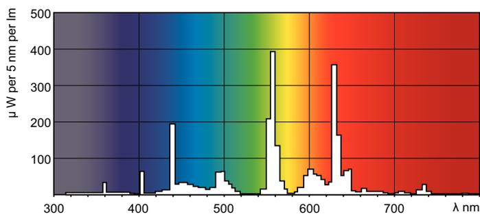
LDPB\_TL-D8ECO\_840-Spectral power distribution B/W
