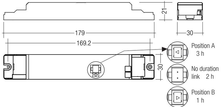
Note: LED Driver supplied with duration link in 3 hours position. Duration link must be set before battery and mains connection. The EM converterLED PRO 134 NiCd is supplied without a duration link. The duration is set to 3 hours and cannot be changed.
