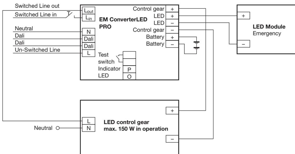
**EM converterLED PRO with a standard LED LED Driver and series operation of LED modules**
