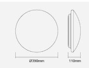
Integrated LED Luminaire F50700SM+IP44
