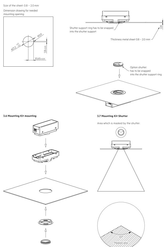
3.8 Wiring and mounting ACU Sensor Housing 14rs IP20
